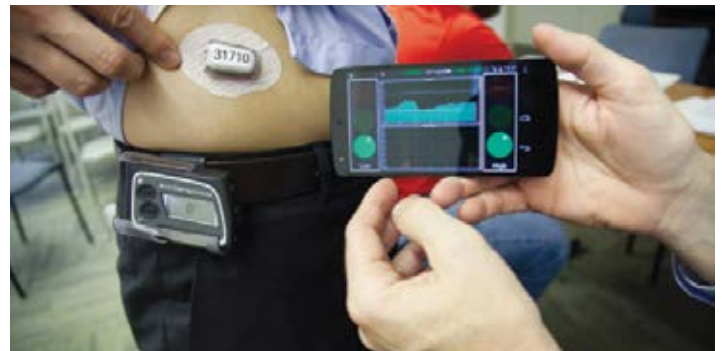
In this early model of an artificial pancreas system, a smartphone communicates with an insulin pump and an implanted glucose sensor to manage and control insulin levels.
