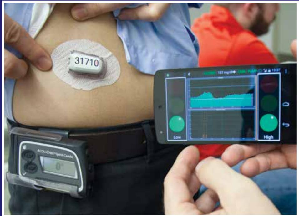
The AP (Artificial Pancreas) system runs an algorithm on a smartphone that communicates with an insulin pump and an implanted glucose sensor.
